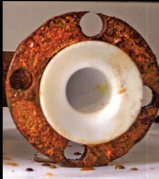
Durcor 2" 90° vs. Carbon Steel 2" 90°
